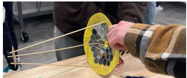
Figure 20. The secondary mirror attached to the primary mirror
