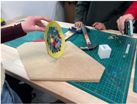
Figure 7. Detached primary mirror and base
